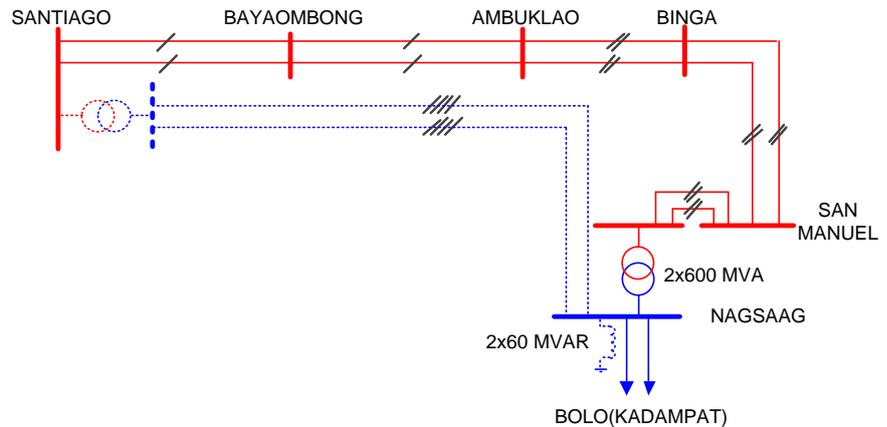
condition of the Santiago–Bayombong and Bayombong–Ambuklao 230 kV Lines. The Project involves the development of a New Santiago 500/230 kV Substation and 140 km 500 kV transmission line from New Santiago going to Nagsaag 500 kV Substation.
