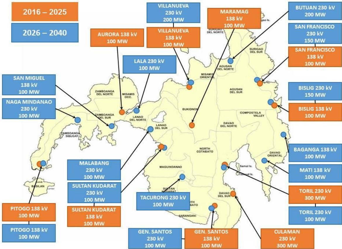
Figure 5.9: Recommended Power Plant Connection Points (Mindanao)
