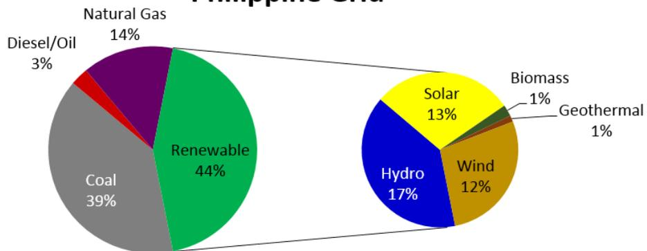
Figure 5.5: Generation Capacity Mix of Indicative Power Plants
