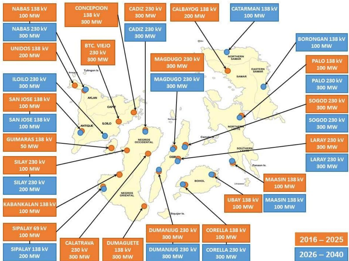
Figure 5.8: Recommended Power Plant Connection Points (Visayas)
