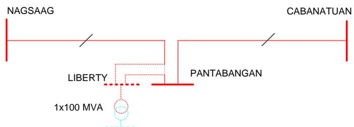
substation will be linked to Nagsaag 230 kV Substation with the development of the Liberty–Nagsaag 230 kV Line.
