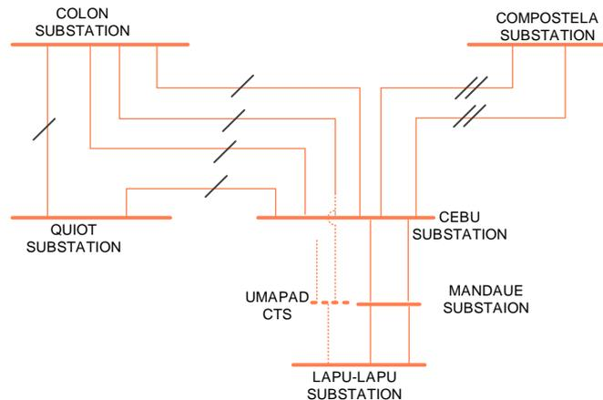
In order to maintain the continuous transmission of power towards the major loads centers in Mandaue and Mactan even during N-1 condition, a new transmission corridor, composed of overhead transmission line and submarine/underground cable system, is proposed between Cebu S/S and Lapu-lapu S/S.
