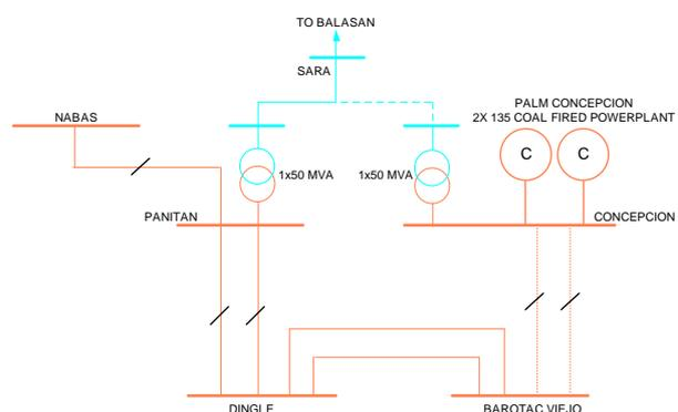
The project involves the construction of a new Concepcion Substation and a 42 km 138 kV double circuit line to Barotac Viejo Substation. Additionally, a 14.2 km 69 kV line will also connect Sara LES to Concepcion Substation, to provide an alternate drawdown for ILECO III.
