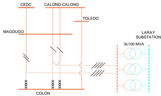
The project will form part of the planned 230 kV transmission loop in Cebu, complementary to the proposed Laray–Naalad 230 kV Energization Project.
