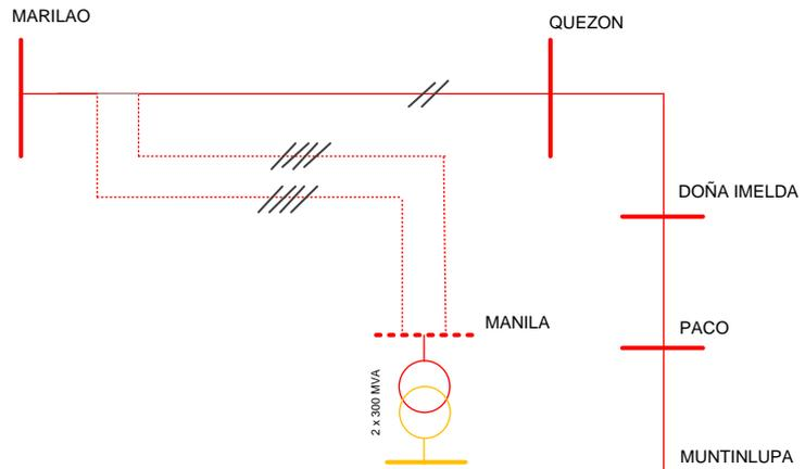
This will expose the Metro Manila loads to supply reliability risk as well as power quality concerns during system peak load condition. The proposed Manila/Navotas 230 kV Substation will be initially linked to the grid through cut-in connection along the existing Marilao-Quezon 230 kV line and will ultimately terminate in the future Marilao 500 kV Substation. The Project will be a Gas Insulated Switchgear (GIS) substation due to the space constraints for an outdoor substation.
