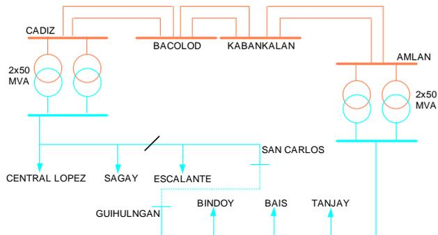
This project involves the construction of a 58 km 69 kV line utilizing a 1-336.4 MCM ACSR conductor from San Carlos to Guihulngan.
