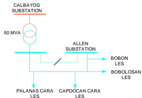
In order to improve the reliability of power delivery towards the northern part of Samar, a 138 kV transmission line (69 kV energized) is proposed which will link Calbayog S/S and the load-end substation in Allen. The project aims to form a loop, thus, will provide single outage contingency to the transmission lines serving Northern Samar.
