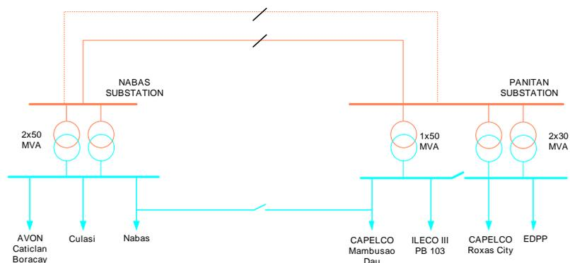
kV line, the 69 kV line will have limited transmission capacity to cater the entire load of the area, hence, will result in power curtailment.
