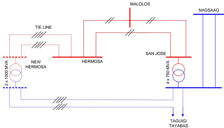
The Project involves the development of new Hermosa 500 kV Substation and construction of a 500 kV transmission line from new Hermosa 500 kV Substation up to San Jose 500 kV Substation. The old Hermosa 230 kV Substation will transfer power through construction of a 230 kV Tie Line to the new Hermosa 500 kV Substation. Shunt Reactors, Line Reactor and Capacitor Banks will also be installed for system voltage regulation during off-peak and peak conditions.
