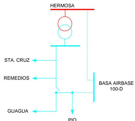
The Hermosa–Floridablanca 69 kV Transmission Line Project involves the construction of a 16.86 kilometer, single-circuit 69 kV transmission line from Hermosa to Floridablanca. Upon implementation of the Hermosa–Floridablanca 69 kV line, PELCO II Sta. Cruz and Remedios will be the only two loads left to the old Hermosa–Guagua line.
