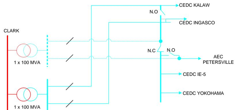
This will address the load growth in the area of Angeles and Mabalacat together with the new industries in Clark Freeport Zone and improve the power quality of supply in the area. The project involves the installation of a new transformer at Clark 230 Substation and the construction of a 69 kV line from the Clark Substation up to the area of Mabiga in Pampanga.
