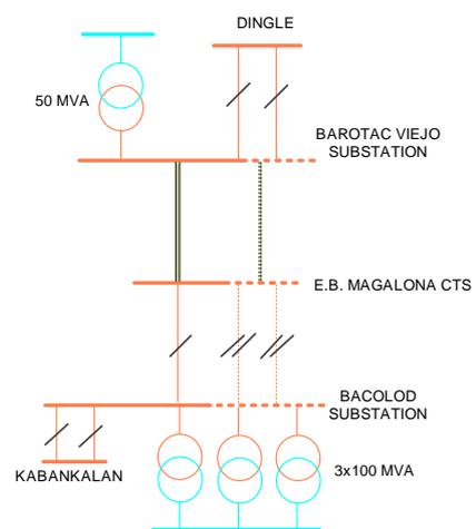
The project involves the development of transmission corridor from Barotac Viejo S/S to Bacolod S/S and will be composed of submarine cable system and overhead transmission lines. It is designed at 230 kV voltage level but will be initially energized and operated at 138 kV. The submarine cable component was already completed in October 2016. The project will also involve associated expansion works at Barotac Viejo and Bacolod Substations.
