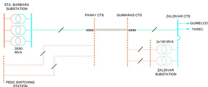
In order to ensure the full dispatch of the San Lorenzo Wind Plant and other prospective generators in the area, it is proposed to energize the Panay-Guimaras Interconnection at 138 kV. The project will also involve the construction of a 2 km overhead line from the cable terminal station in Panay towards PEDC substation, as well as the expansion and upgrading works at Zaldivar S/S and PEDC S/S.
