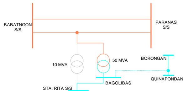
This project involves the construction of a 103 km 69 kV line connecting Sta. Rita and Quinapondan Substations.
