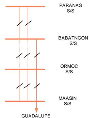
This project involves the construction of a 78.54 km of 138 kV steel tower overhead transmission line utilizing 1-795 MCM ACSR conductor as second circuit of the existing Ormoc – Babatngon 138 kV Line. This project also involves the expansion of Ormoc and Babatngon Substations.
