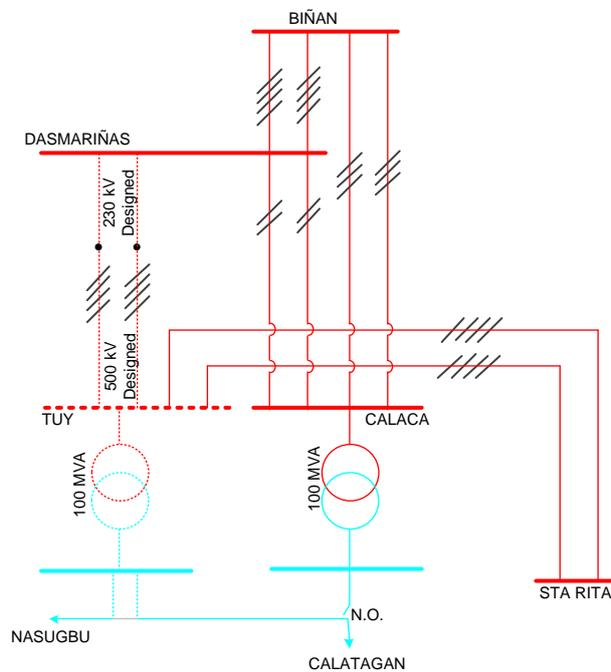
The Tuy 500 kV Substation (Stage 1) Project will involve the development of Tuy 500 kV Substation which will be initially energized at 230 kV voltage level. The project will also involve the development of Tuy–Dasmariñas 500 kV designed transmission line but will also be initially energized at 230 kV. Furthermore, a new 100 MVA, 230/69-13.8 kV Power Transformer will be installed to provide N-1 contingency to the existing 100 MVA Power Transformer at Calaca Substation.
