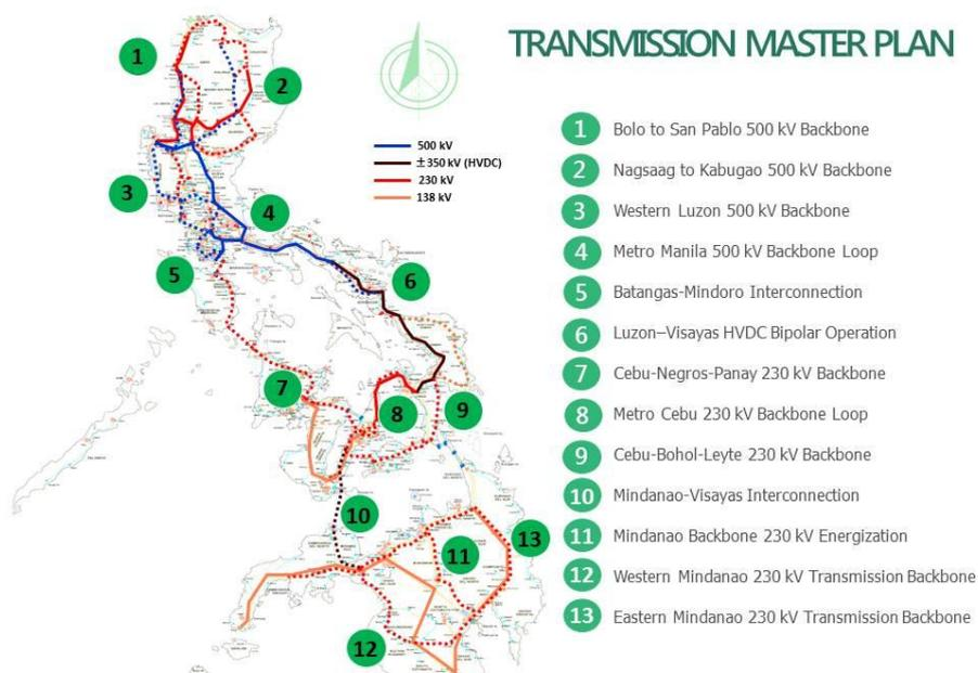
Figure 11.1 - Transmission Backbones and Island Interconnections
